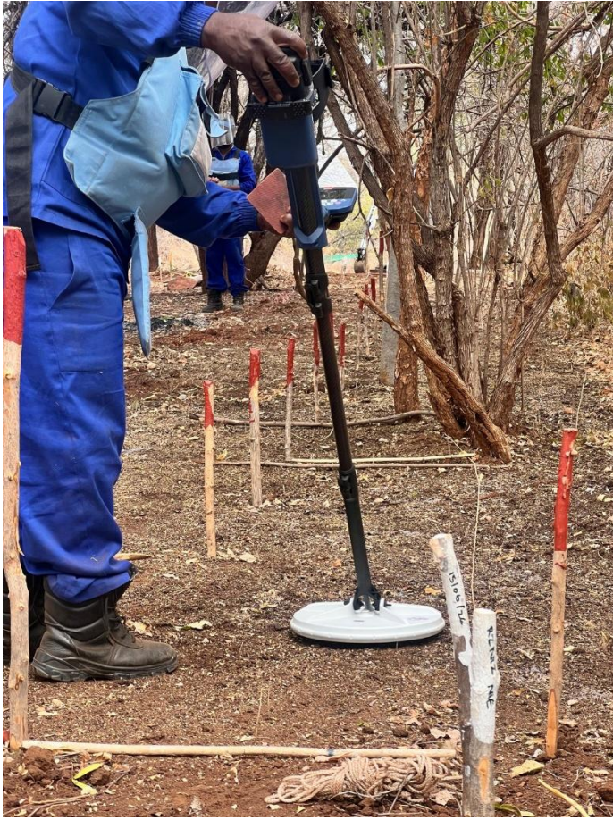
Pictured Below: The GPZ detectors in use in the minefield
